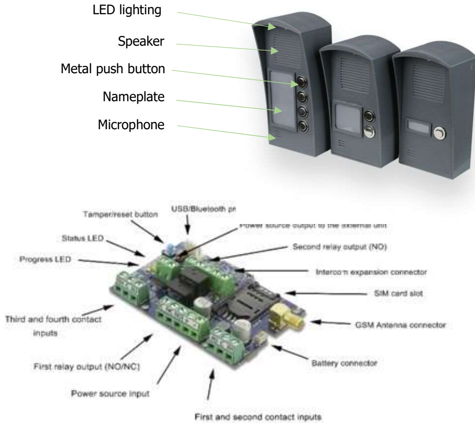
Figure 2: the buildup of the module
